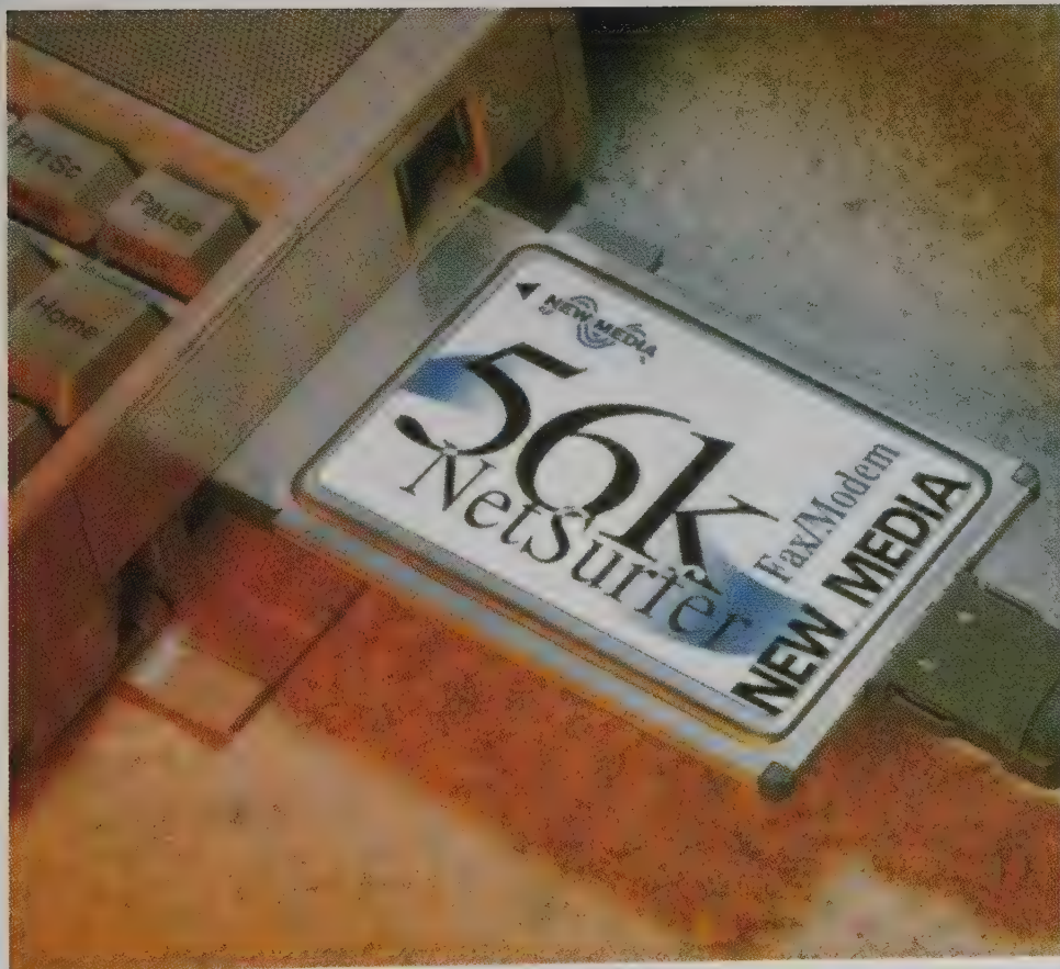
FIGURE 4.6 Slots for PCMCIA Cards Expand the Capabilities of Laptops and Notebooks
