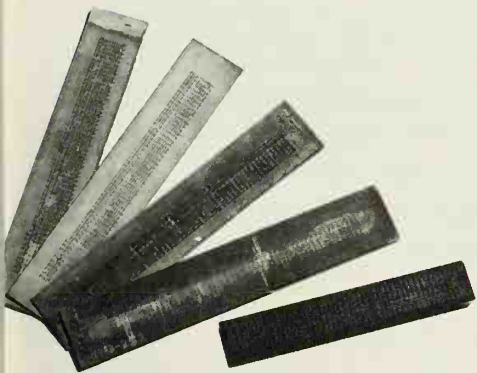
An assortment of printing molds produced by the second Difference Engine. The molds are made by the flat, perpendicular gadget in the center.
