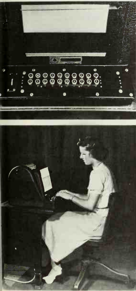
The Model I took its instructions from any of three modified teletypes, although it could be used by only one person at a time.
