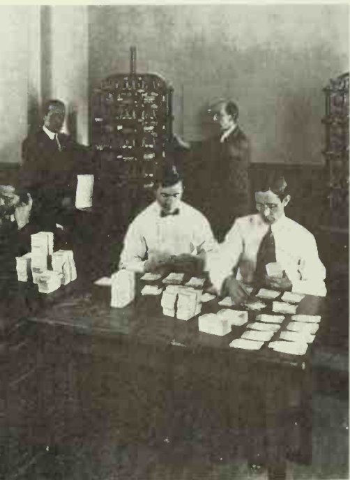
In 1894, John K. Gore, an actuary for the Prudential Insurance Company, patented an automatic punch card sorter (in the background). It consisted of four circular platforms, each containing ten bins configured with a different arrangement of pins. A motor turned the platforms, and the cards dropped into the appropriate bins. Although Gore's invention could process about 15,000 cards an hour, it was built with Prudential needs in mind and wasn't used elsewhere.
