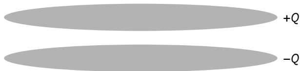
Figure 3.6 Two parallel plates form a capacitor.
