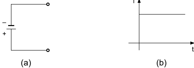
Fig. 9.1. A direct current source (a) and current versus time (b).
